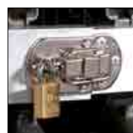
Lockable metal bar to secure the guns
